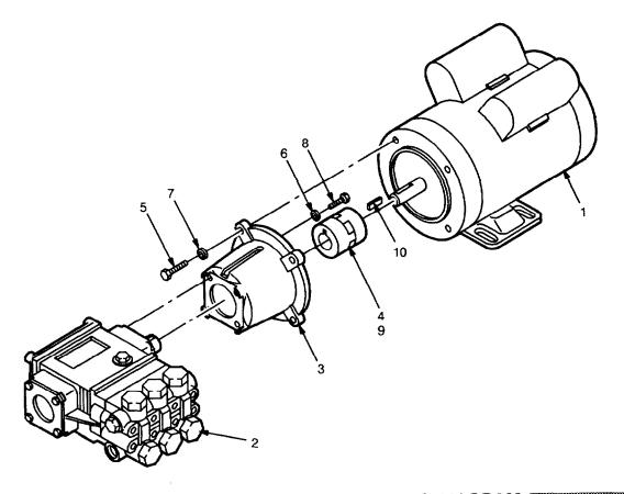
PARTS LIST 800-248 Pump and Motor Assembly
